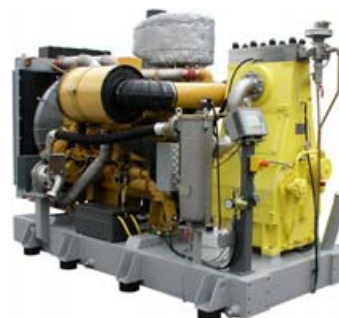
Typical high pressure pump units
