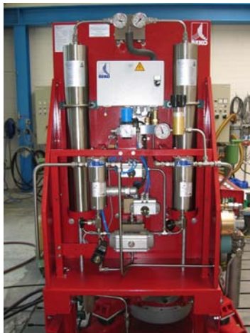
AKER KVAERNER WP5000 Air Compressor
