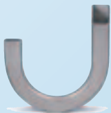
Oval pipe 30 x 15 x 2 mm, bent on TUBOMAT 642
