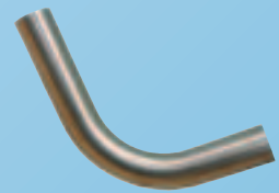
Stainless steel pipe 76,1 x 1,5 mm, bent on TUBOTRON 90
