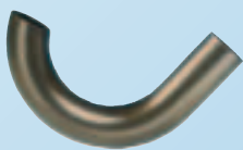
CuNiFe pipe 42 x 2 mm, bent on TUBOTRON 50
